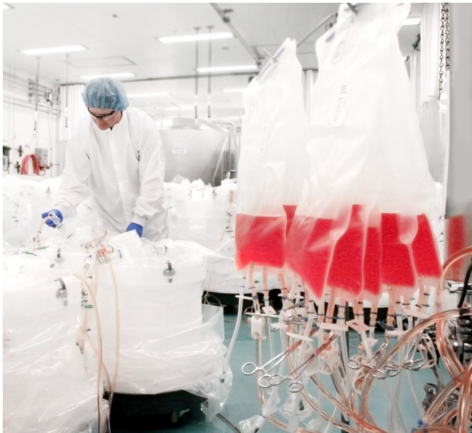
Fig 1. Filling 2D bags with HyClone cell culture media.
