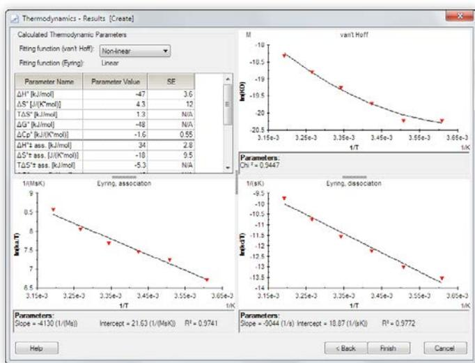
**Fig 12.** Automatic generation of Eyring and van't Hoff plots from kinetic data for calculation of the thermodynamic parameters.
