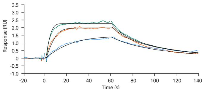
**Fig 3.** Binding of a small molecule, xanthine amine congener (XAC), to stabilized histidine-tagged GPCR (Star™) A2. Data of higher quality is generated by Biacore™ T200 (lower sensorgram) compared to Biacore™ T100 (upper sensorgram) when using low levels of immobilized GPCR. Data courtesy of Dr. Andrei Zhukov, Heptares Therapeutics Ltd, Welwyn Garden City, UK.
