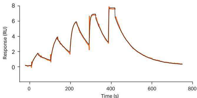
**Fig 8.** Using the single-cycle kinetics approach, samples are injected one after the other in the same cycle with no intervening regeneration steps. Here, a dilution series of a molecule with a relative molecular mass ( $M_r$ ) of 312 was prepared at concentrations of 0.062, 0.185, 0.556, 1.667, and 5  $\mu\text{M}$ , and sequentially injected over a sensor surface prepared with a protein ( $M_r$  29 000) immobilized at 760 RU.
