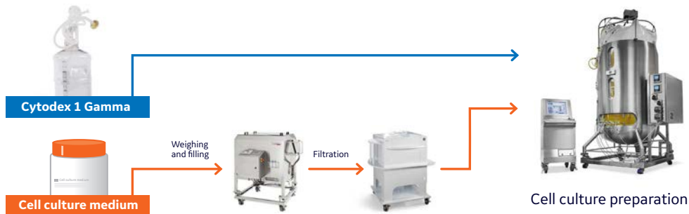
Fig 4. Assumed preparation procedure for Cytodex 1 Gamma microcarriers at 500 L scale.
