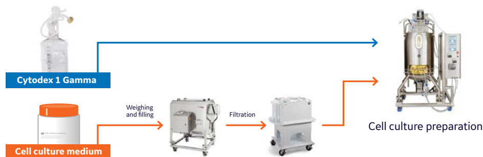
Fig 2. Assumed preparation procedure for Cytodex 1 Gamma microcarriers at 100 L scale.
