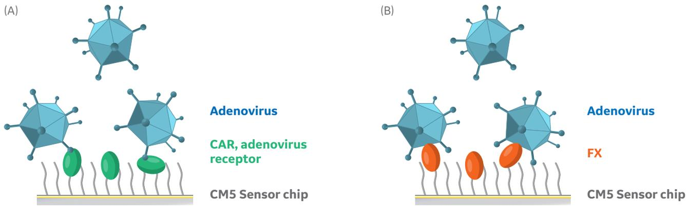
**Fig 2.** Principle of the two Biacore assays for determination of adenovirus concentration, where virus particles injected in a flow system bind to (A) the CAR receptor via the virus fiber protein or (B) FX via the virus hexon protein. In the separate assays, CAR or FX protein is immobilized on Sensor Chip CM5, and bound virus is detected using the Biacore T200 system.
